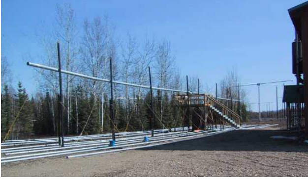
Fig. 1. Photograph (April 2003) of the 2.85-MHz (18-cm diameter – 5200 cm long) Hertzian antenna at HIPAS, suspended from insulating 10-cm diameter ABS drainpipes, 500 cm above a ground plane made up of 6.4-cm diameter aluminum pipes. The antenna has a capacitance of 200 pF across its central spark gap. The stairways are for central access. One of the antennas of the CW array at HIPAS can be seen in the background. The north side of the Generator Building is on the right side of the picture.
