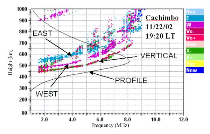
**Fig. 3.** Multi-directional ionogram at Cachimbo for 22 November at 19:20 LT showing echo traces from the west, east, and overhead, with an overlay of the vertical electron density (plasma frequency) profile.
