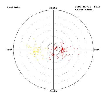
**Fig. 4.** Cachimbo skymap for 22 November at 19:13 LT showing echoes from the west with Doppler frequencies of -0.5 Hz, and from the east with Doppler frequencies of -2.0 Hz. The skymap displays zenith angles from 0 to  $20^{\circ}$ .
