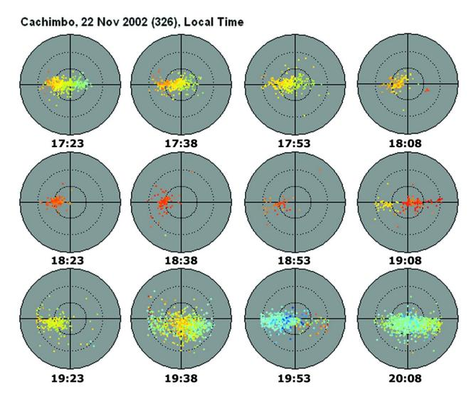
Fig. 5. Skymaps for Cachimbo on 22 November from 17:23 LT to 20:08 LT, showing the effect of the terminator passing at ∼18:00 LT.
