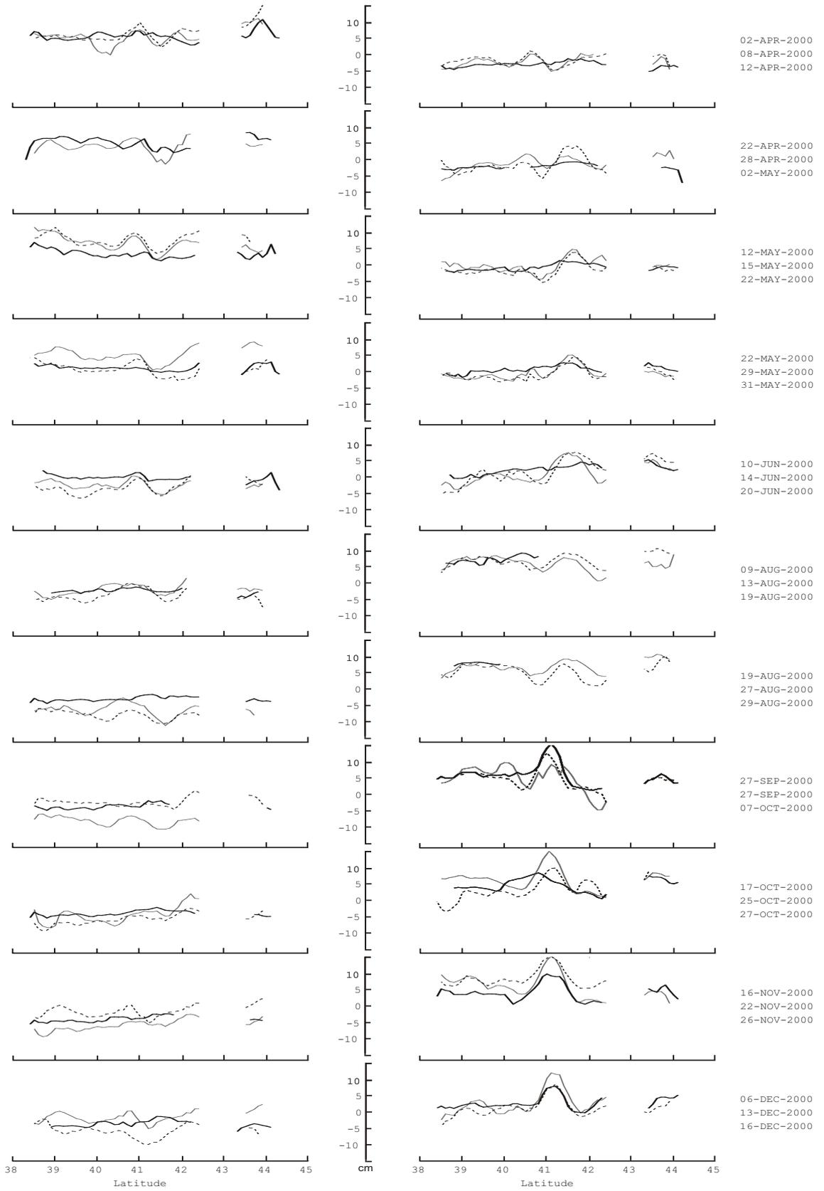
**Fig. 6.** XBT steric heights relative to 300 m for the 22 cruises (tick solid line). Dashed (shaded) lines are the altimetric heights before (after) the time frame of the cruise. The horizontal axis is latitude (degrees).
