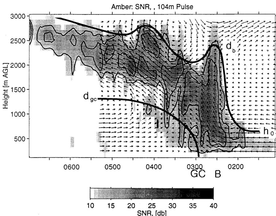
**Fig. 9.** Two-dimensional flow field relative to motion of the gravity current derived from the Amber, Oklahoma, UHF wind profiler for 0100–0515 UTC 17 April, 1991, and signal-to-noise ratio from the vertical beam. For definitions of the curves and other notations, see Koch and Clark (1999)
